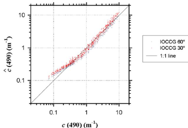
**Figure 7.** Relationship between the estimated beam attenuation coefficient  $\hat{c}(490)$  and the measured  $c(490)$  for the synthetic IOCCG data set. The estimates of  $\hat{c}(490)$  were obtained with the nominal version of the algorithms using two reflectance bands as inputs,  $R(490)$  and  $R(709)$  and the determination coefficient  $R^2$  is 0.97.
