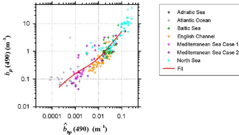
**Figure 1.** Relationship between the measured particle scattering coefficient at 490 nm  $b_p(490)$  and the estimated particle backscattering coefficient at 490 nm  $\hat{b}_{bp}(490)$  for the in situ COASTIOOC data set. The estimates of  $\hat{b}_{bp}(490)$  were obtained with the nominal version of the algorithms using two reflectance bands as inputs,  $R(490)$  and  $R(709)$ .
