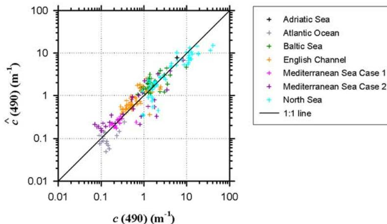
**Figure 4.** Relationship between the estimated beam attenuation coefficient  $\hat{c}(490)$  and the measured  $c(490)$  for the in situ COASTIOOC data set. The estimates of  $\hat{c}(490)$  were obtained with the nominal version of the algorithms using two reflectance bands as inputs,  $R(490)$  and  $R(709)$ , and the determination coefficient  $R^2$  is 0.86.
