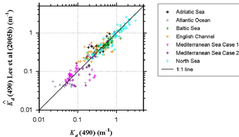
**Figure 10.** Relationship between the estimated vertical diffuse attenuation coefficient  $\hat{K}_d(490)$  and the measured  $K_d(490)$  for the in situ COASTIOOC data set. Estimates of  $\hat{K}_d(490)$  were obtained with the algorithms proposed by Lee *et al.* [2002, 2005a, 2005b]. The determination coefficient  $R^2$  is 0.87.
