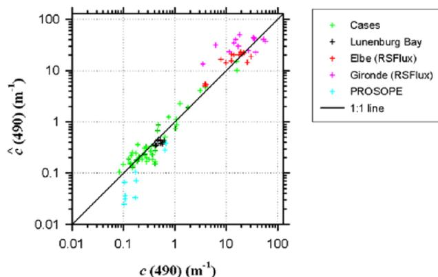
**Figure 9.** Relationship between the estimated beam attenuation coefficient  $\hat{c}(490)$  and the measured  $c(490)$  for the CASES, Lunenburg Bay, RSFlux, and PROSOPE data sets. Estimates of  $\hat{c}(490)$  were obtained with the nominal version of the algorithms using two reflectance bands as inputs,  $R(490)$  and  $R(709)$ , and the determination coefficient is 0.95.
