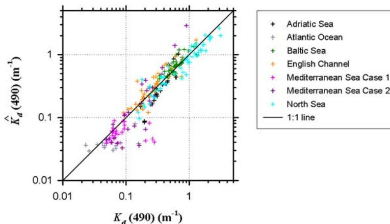
**Figure 3.** Relationship between the estimated vertical diffuse attenuation coefficient  $\hat{K}_d(490)$  and the measured  $K_d(490)$  for the in situ COASTIOOC data set. The estimates of  $\hat{K}_d(490)$  were obtained with the nominal version of the algorithms using two reflectance bands as inputs,  $R(490)$  and  $R(709)$ , and the determination coefficient  $R^2$  is 0.88.
