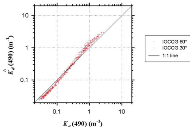
**Figure 6.** Relationship between the estimated vertical diffuse attenuation coefficient  $\hat{K}_d(490)$  and the measured  $K_d(490)$  for the synthetic IOCCG data set. The estimates of  $\hat{K}_d(490)$  were obtained with the nominal version of the algorithms using two reflectance bands as inputs,  $R(490)$  and  $R(710)$ , and the determination coefficient  $R^2$  is 0.99.
