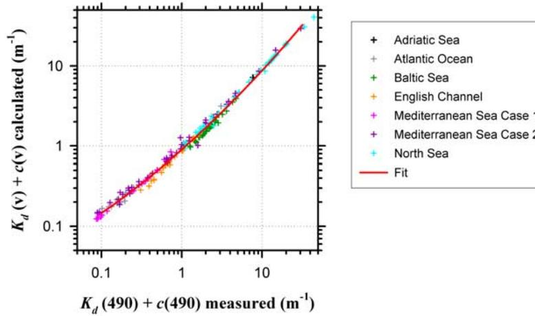
**Figure 2.** Relationship between the sum of the visual attenuation coefficient and the visual beam attenuation coefficient  $K_d(v) + c(v)$  versus the measured vertical attenuation coefficient and the beam attenuation coefficient at 490 nm  $K_d(490) + c(490)$  for the in situ COASTIOOC data set. The fit is quadratic polynomial.
